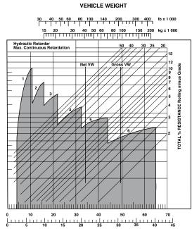
**Instructions:** From intersection of Vehicle Weight with Percentage Resistance line read across to determine maximum Gear attainable, and then downwards for Vehicle Speed.
